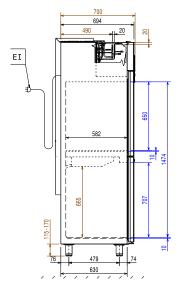
Electrical inlet (power) ΕI Refrigerant Inlet RO Refrigerant Outlet
